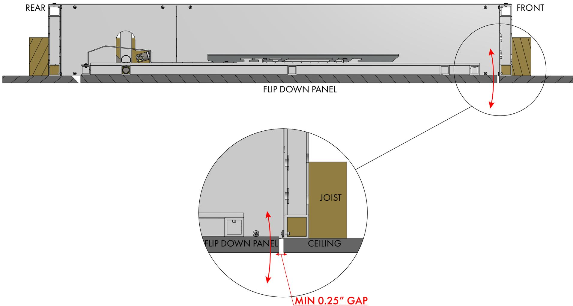
CEILING PANEL MUST BE ABLE TO RAISE INTO FRAME WITHOUT OBSTRUCTION
