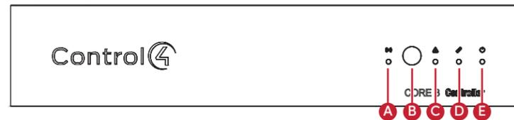
**A Activity LED**—The Activity LED shows when the controller is streaming audio.
